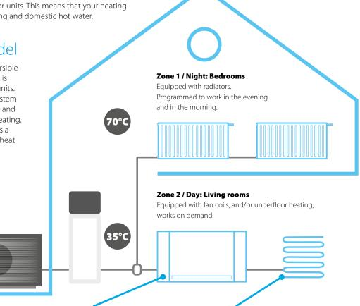
**Heat pump convectors** are hydronic emitters that can provide cooling or heating. They can be combined and are a perfect fit with underfloor systems.
